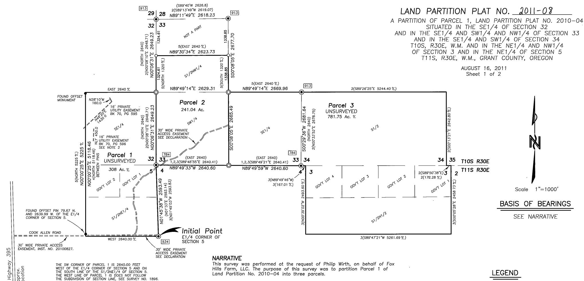
1) The unsurveyed section lines and subdivision of section lines are protracted and the parcel dimensions are approximate. The actual boundary dimensions will conform to the description given in the Surveyor's Certificate.
