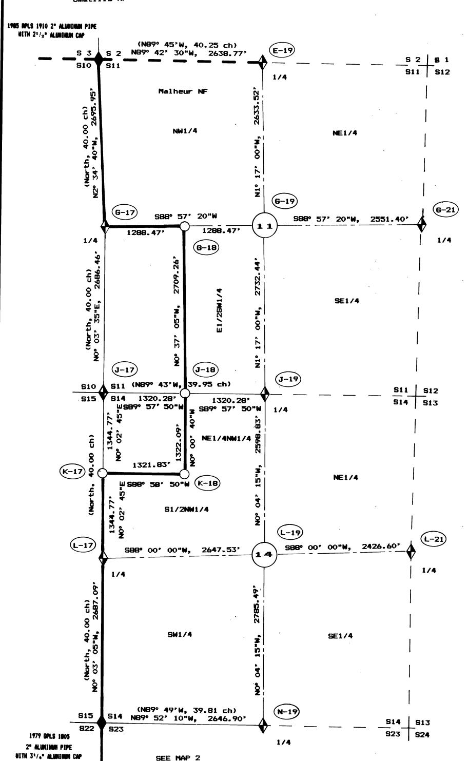
LEGEND Section Corners Previously Set Section & 1/4 Corners Set by Found Evidence C1/4 Corners Set by Survey 1/16 Corners Set by Survey Posted National Forest Boundary Lines NF Boundary Not Posted This Survey Section Lines Center Section Lines Basis for Bearings Solar Observation Projected Lines Assumed Magnetic Declination 18° 30'E Legal Subdivision of USFS Property S1/2NW1/4 400' B00' 1600' Record Bearing & Distance in Parentheses (North, 40.00 ch)
