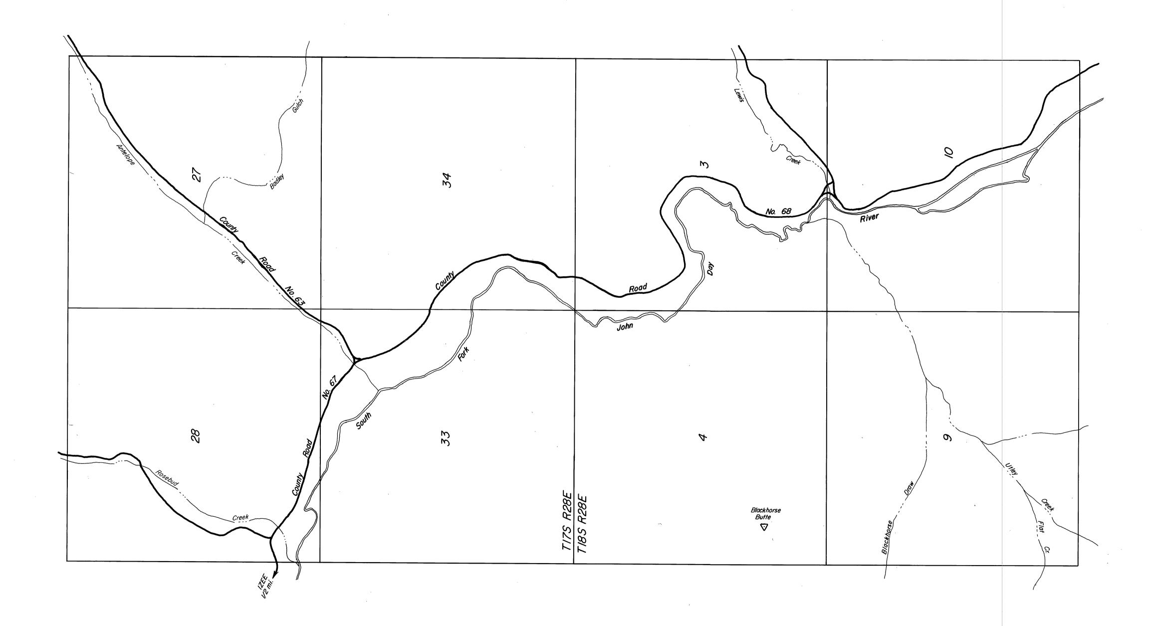
NARRATIVE: This survey was performed at the request of the Grant County Roadmaster to establish the right-of-way for the lower portion of County A search was made of the available records pertaining to this survey. I find no deeded right-of-way on this portion of the road. right-of-way lines as shown hereon.
