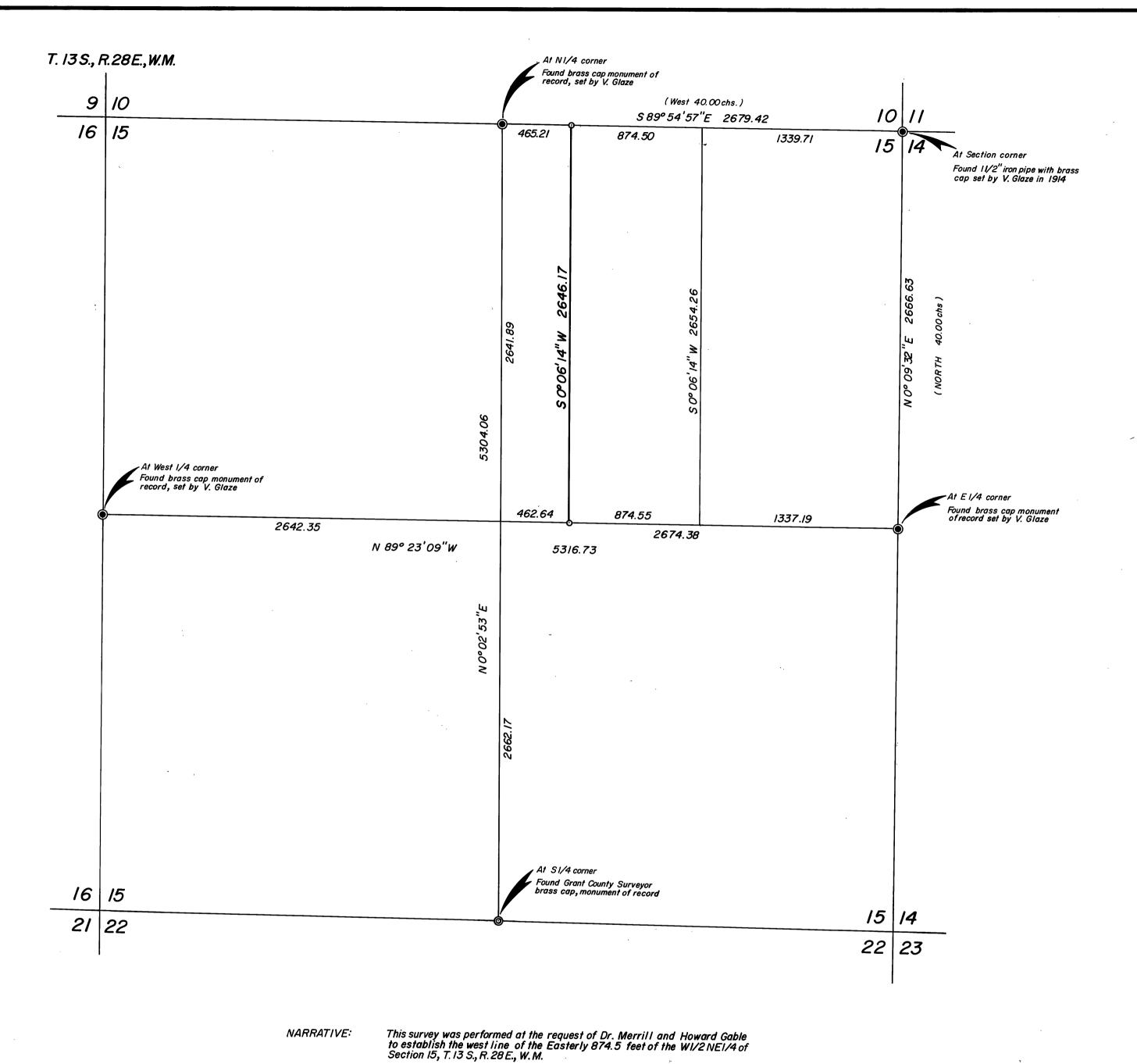
A search was made of the available records pertaining to this survey. Field measurements were made to locate existing monuments. New monuments were set in accordance with the evidence found.
