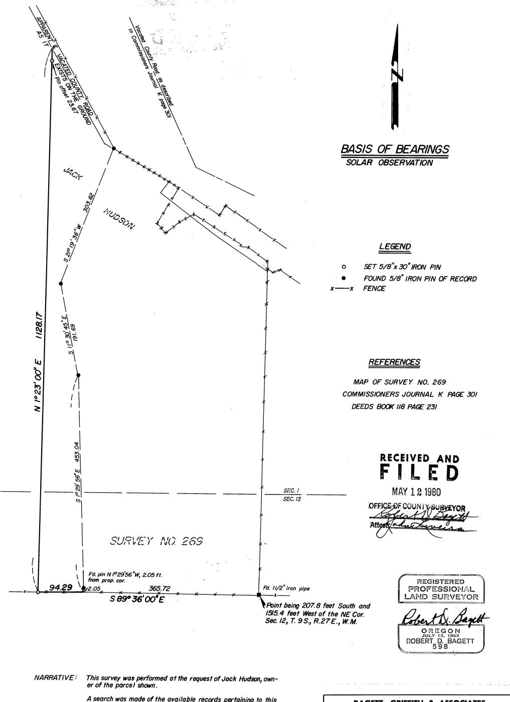
A search was made of the available records pertaining to this survey. Field measurements were made to locate existing monuments. New monuments were set in accordance with the evid-ence found. The vacated County Road as it exists on the ground is substantially different from wherethe centerline description in the vacation document places it. This difference is shown chove above.
