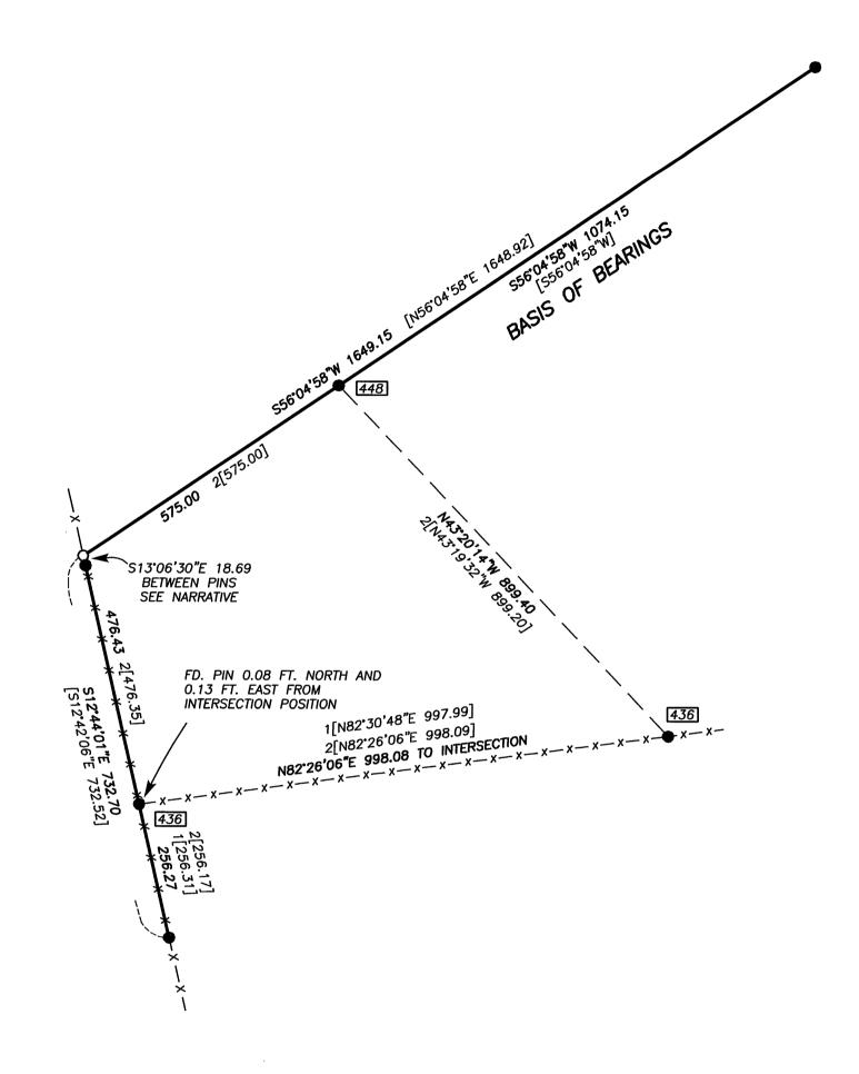
THE PURPOSE OF THIS SURVEY IS TO SET AN IRON PIN AT THE CORRECT LOCATION AS SHOWN ON RECORD MAP OF SURVEY NO. 410. WE MADE FIELD MEASUREMENTS TO LOCATE APPURTENANT MONUMENTS SHOWN ON RECORD MAP OF SURVEY NO. 410, 436 AND 448, AS SHOWN.
