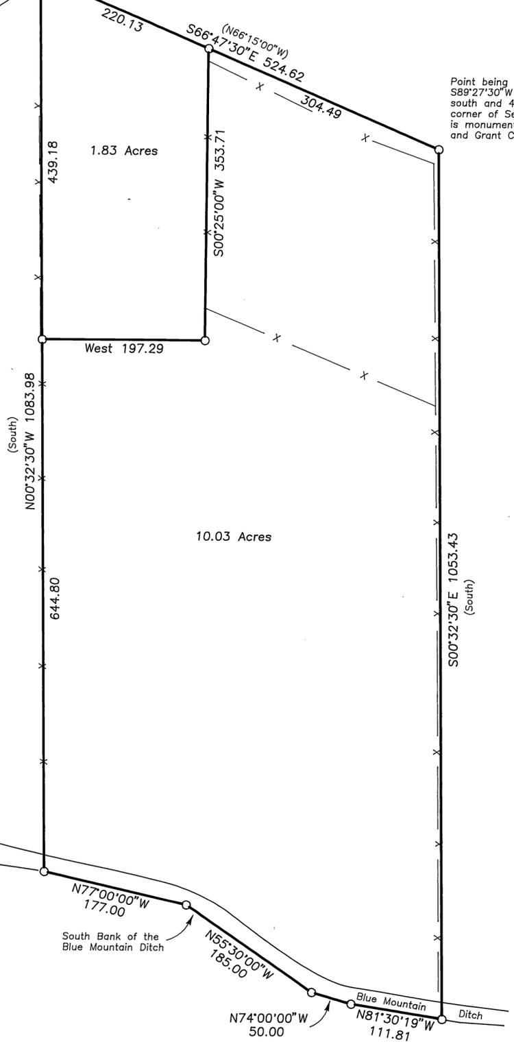
Point being  $S00^{\circ}32'30''E$  1006.00' and  $S89^{\circ}27'30''W$  481.90', record is 1006.0' south and 481.90' west, from the NE corner of Section 30. The section corner is monumented with a  $1\frac{1}{2}''$  iron pipe and Grant County Surveyor brass cap.
