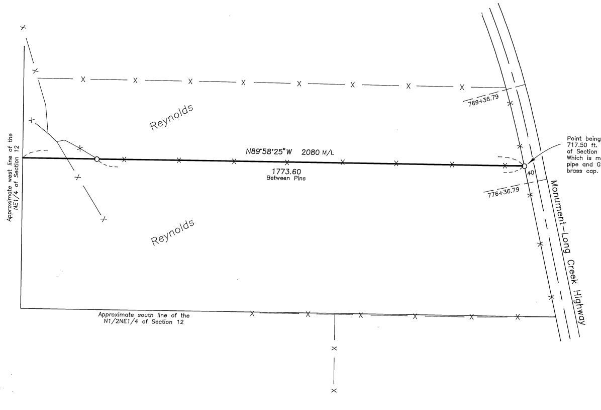
Point being 697.20 ft. South and 717.50 ft. West of the NE corner of Section 12, T9S, R27E, W.M. Which is monumented with a 1½" iron pipe and Grant County Surveyor
