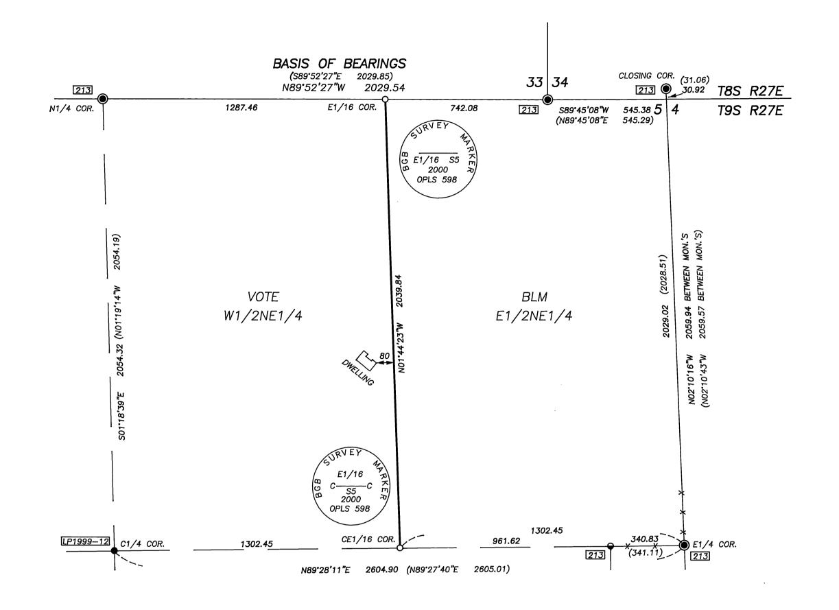
THIS SURVEY WAS PERFORMED AT THE REQUEST OF LARRY VOTE. THE PURPOSE OF THIS SURVEY WAS TO LOCATE AND MONUMENT THE NE AND SE CORNERS OF THE W1/2NE1/4 OF SECTION 5, T.9 S., R.27 E.
