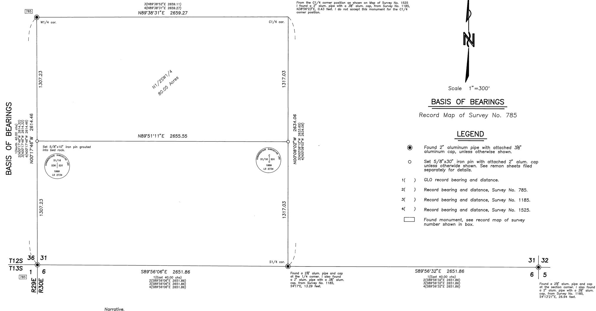
This survey was performed at the request of Tom Thomsen. The purpose of this survey was to establish the south line of the N1/2SW1/4 of Section 31, as shown.
