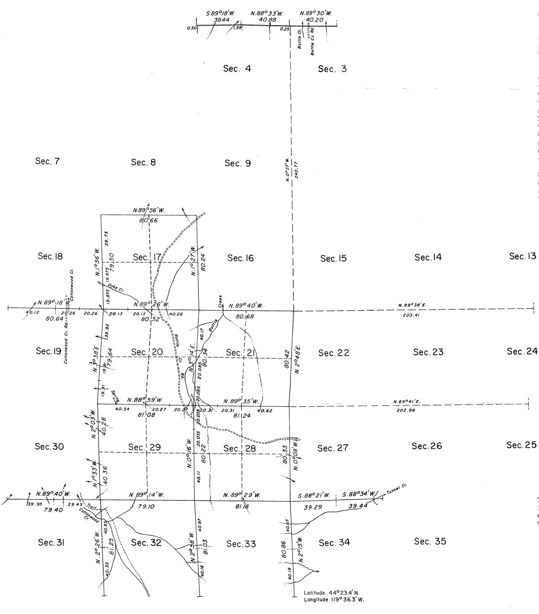
This plat represents a retracement and reestablishment of a portion of the Third Standard Parallel South, south boundary of T. 12 S., R. 26 E., and a portion of the subdivisional lines, designed to restore the corners in their true original locations according to the best available evidence. Areas are as shown on the plat approved December 1, 1873.
