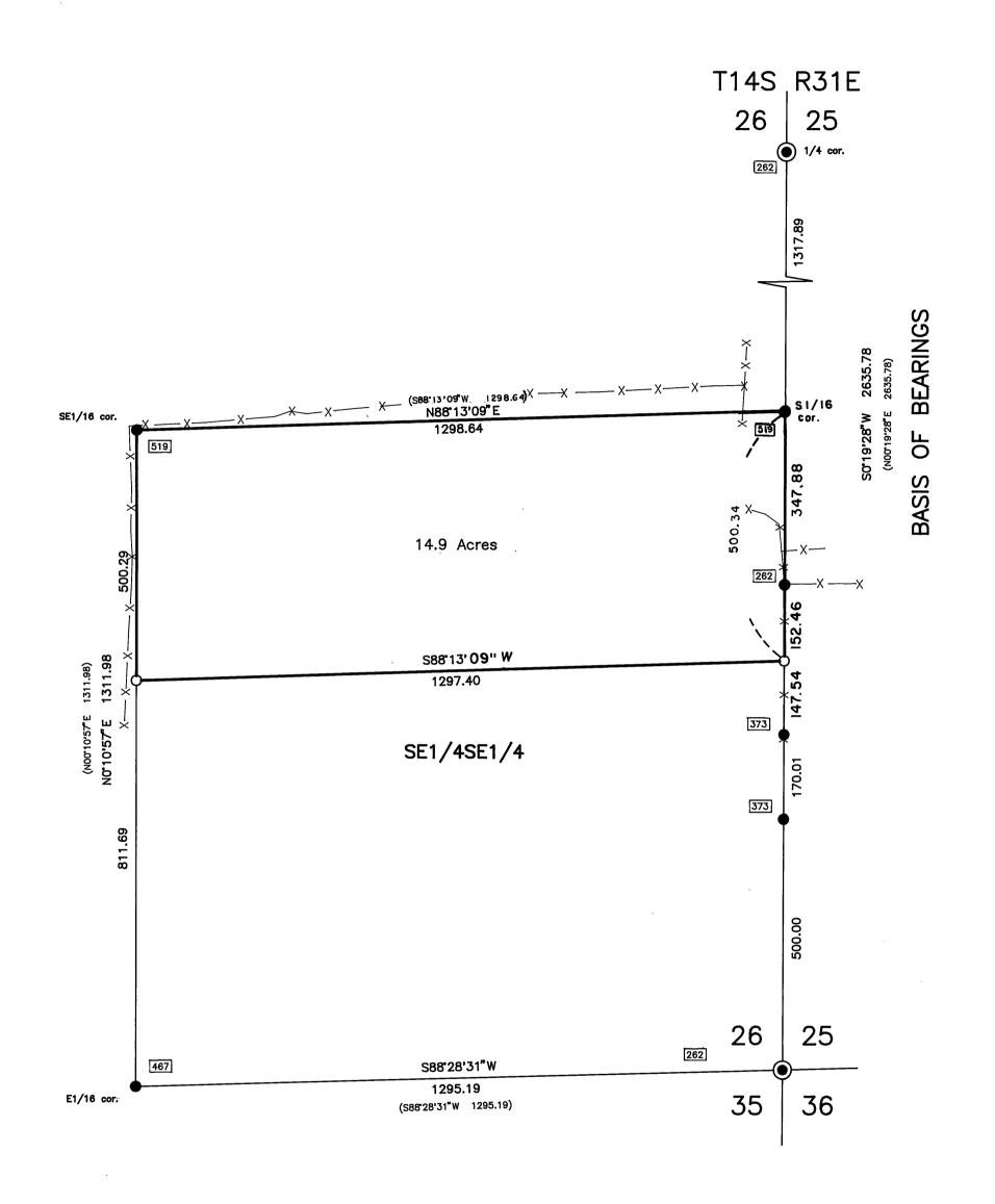
NARRATIVE: This survey was performed at the request of Monte Thissell, Dana Jennings and David Kirk, The purpose of this survey was to locate the north 500 feet of the SE1/4SE1/4 of Section 26, and to mark the boundary lines with lath and flagging, as shown hereon.
