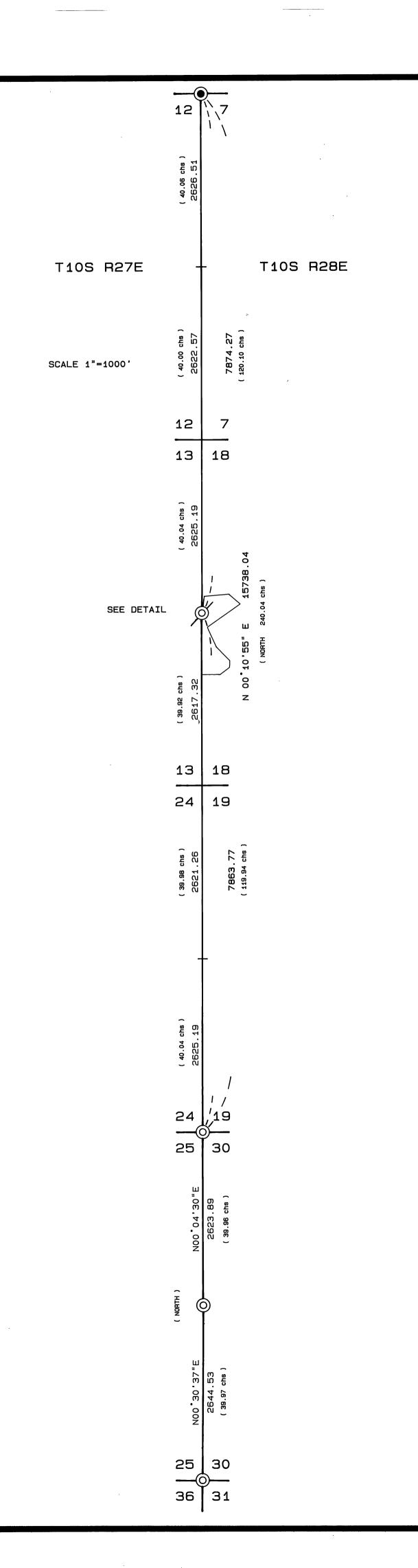
DETAIL T10S R27E T10S R28E SEC.13 SEC.18 N85 17 53 E ROCK QUARRY SITE GOV'T LOT 2 GOV'T LOT 3 NOTE: We drove 6 ft. long galvanized steel fence posts alongside each pin set. Existing Crushed CRUSHED ROCK STORAGE SITE 4.61 Acres
