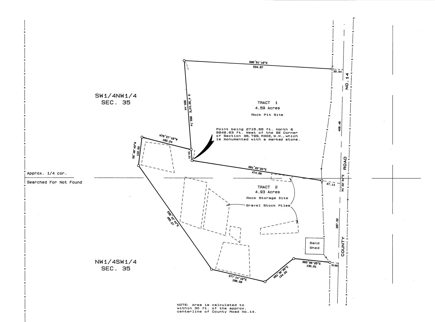
NARRATIVE: This survey was performed at the request of Ab Bezona, County Road Supervisor. The purpose of this survey was to delineate an area for a rock pit and rock storage site.
